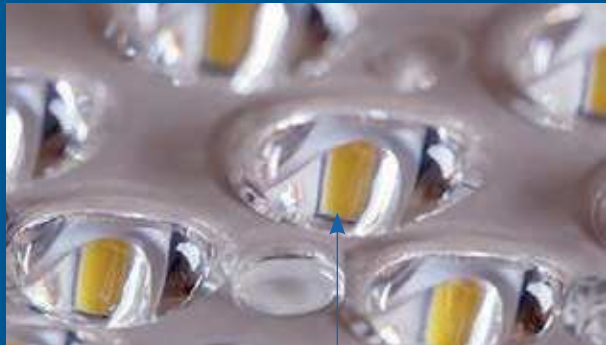
Conventional optic with single LED image (yellow)
