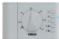
02900.1 Electronic thermostat for ON/OFF ambient temperature control (heating and air-conditioning), class I temperature control device (contribution 1%), change-over relay output 5(2) A 240 V~, AA LR6 1,5 V battery-powered (not supplied), surface mounting, white
