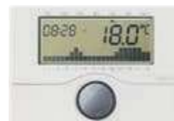
01910 Electronic timer-thermostat for ON/OFF ambient temperature control (heating and air-conditioning), daily/weekly programming, class I temperature control device (contribution 1%), change-over relay output 5(2) A 250 V~, AA LR6 1,5 V battery-powered (not supplied), surface mounting, white
