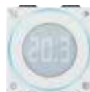
09470 Rotary dial thermostat for ambient temperature control, 5(2) A 240 V~ relay output, heating and air-conditioning ON/OFF, class I temperature control device (contribution 1%) in ON/OFF mode, white LED backlighting and brightness regulation, 100-240 V 50/60 Hz - 2 modules. Depth: 28,5 mm
