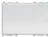
■ 14453 Transponder card reader with vertical pocket for installation inside rooms, KNX standard, 2 NO 4 A 24 V~ relay outputs, 2 inputs, supplementary power supply 12-24 V~ 50/60 Hz and 12-24 Vdc (SELV) - 3 modules
