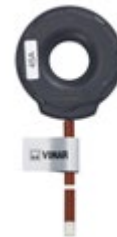
01458 Toroidal current sensor for load control and power measurement, hole diameter 19 mm, cable length 40 cm
