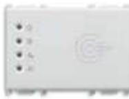
■ 14457 Transponder card reader for installation outside rooms, KNX standard, 2 NO 4 A 24 V~ relay outputs, 2 inputs, power supply 12-24 V~ 50/60 Hz and 12-24 Vdc (SELV) - 3 modules. Supplied without transponder card
