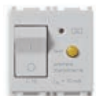
14411.10.SL C 10, I_{\Delta n} 10 mA prekidna moć 3000 A - 2 modula. Dubina: 38 mm
