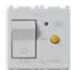
14411.16.6.SL C 16, I_{\Delta n} 6 mA prekidna moć 3000 A - 2 modula. Dubina: 38 mm
